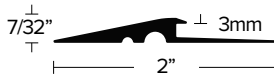
LVT 113 LVT Reducer TRANSITIONS FROM 3MM LVT TO ZERO. FINISH: EA, EN, BRZ
